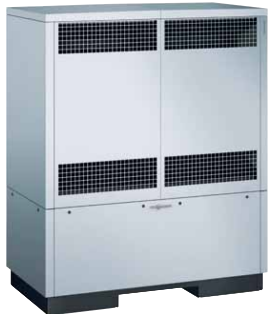
Vitocal 300-A (AWO 302.B60) The Vitocal 300-A from Viessmann is an air source heat pump in the output range from 13.2 to 55.8 kW. With a cascade of up to five Vitocal 300-A heat pumps, an output of up to 279 kW is possible.
